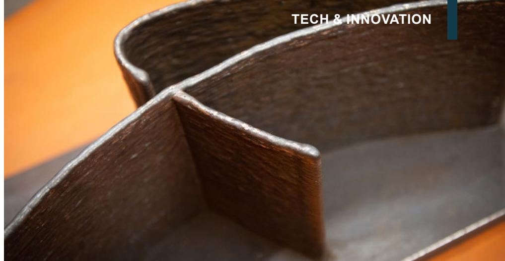
A study which has been performed by Guaranteed in close collaboration with DNV and Kongsberg Maritime, a comparative life cycle analysis was made for several parts. As compared to conventional manufacturing options such as casting or forging, the results of this study clearly demonstrate the significant savings which can be achieved in terms of carbon emissions and energy consumption for WAAM production and even more so for WAAM repair or refurbishment.
