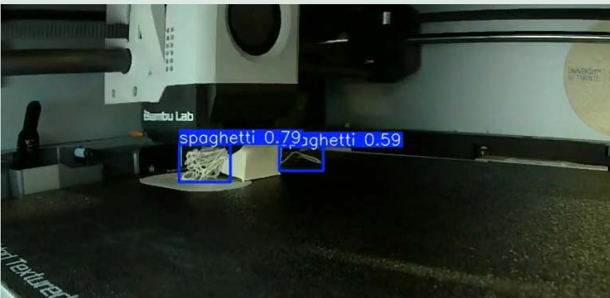
▲ Figure 3. YOLO11 output, showing two detected spaghetti defects.
