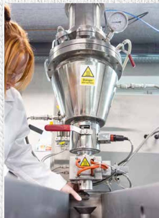
► For wet spinning, the polymer solution needs to be passed through a spinneret.
