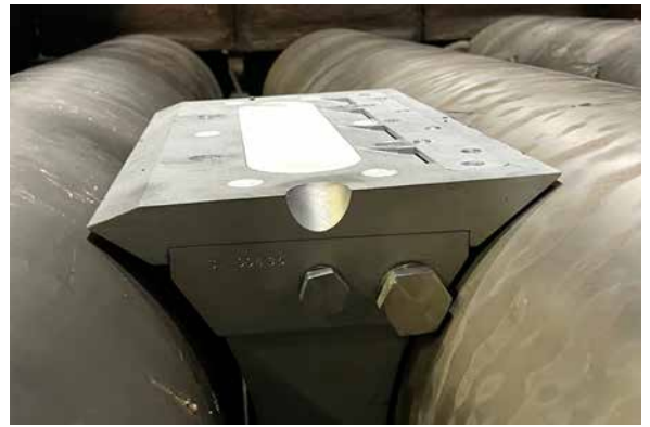
Figure 3: Phase transformation sensor operational in the hot strip mill.
