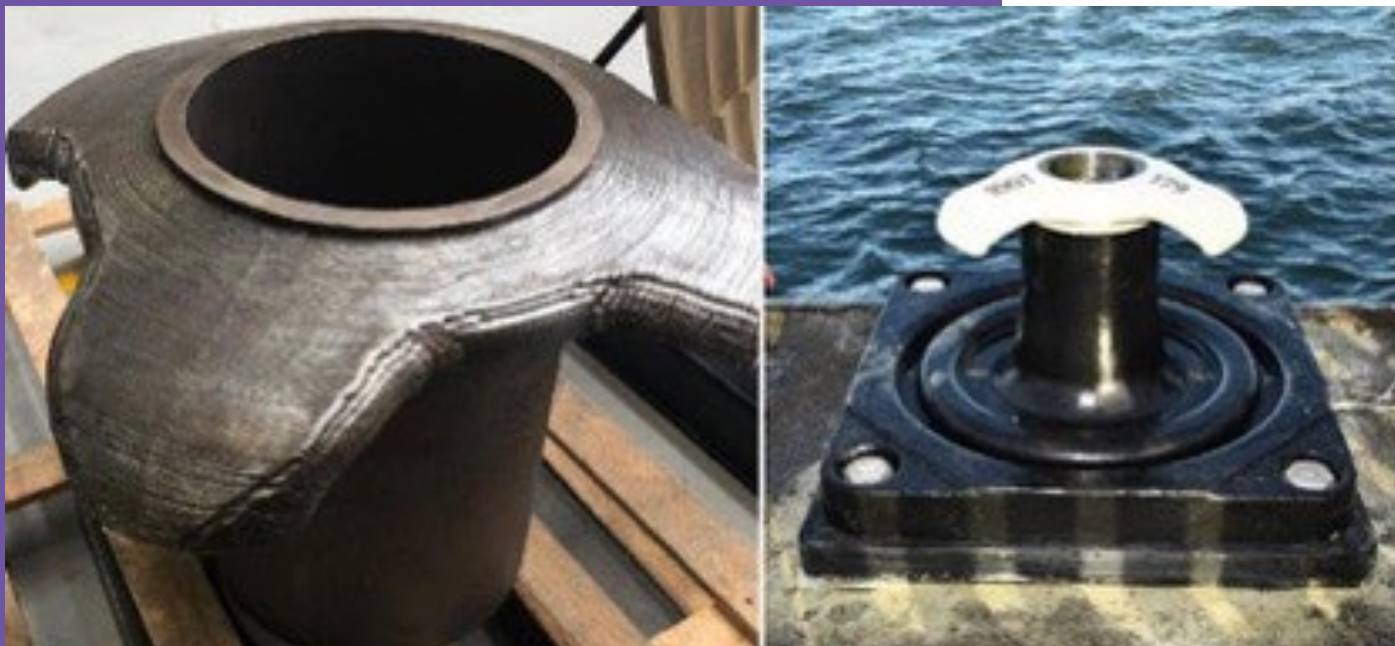
▲ Figure 2 examples on the left: WAAM 3D printed Bolder; on the right: smart bolder in the Rotterdam region.
