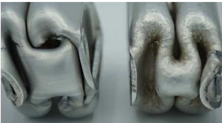
◀ Crash deformation simulation of Al-parts, left broken, right only deformed!
