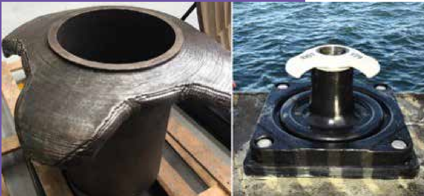
▲ Figure 2 examples on the left: WAAM 3D printed Bolder ; on the right: smart bolder in the Rotterdam region .
