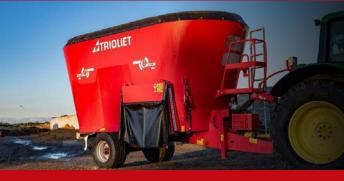
The Shifttronic makes it possible for the heavier machines (>18m3) to be driven by lighter tractors. The Shifttronic switches automatically to the most appropriate mixing speed. This prevents overloading in the drive line of the mixer feeder and of the power take off of the tractor, and requires less power.
