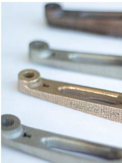
*Comparative testing of different metal Additive Manufacturing Technologies and materials for a bike pedal arm.*
